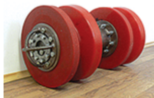
VOSTOK-MD cup-and-disk pig with front-mounted VOSTOK-VR recorder installed before the testing.
